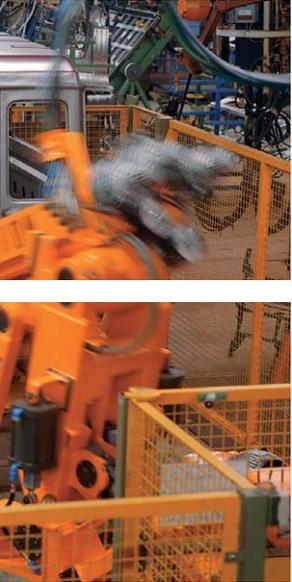
Solenoid interlocks demand accurate alignment of actuator and device. This requirement is met on new machinery. But during its lifetime, the situation may occur in which the actuator can no longer easily enter the device. As a consequence, both parts become damaged. This in turn leads to machine downtime and repair costs.
