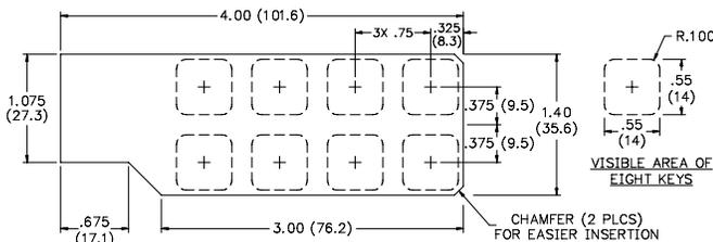
When inserting the key strip into the slot in the G303 panel, start one corner first then slowly insert the strip into place.
