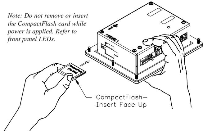
Information stored on a CompactFlash card by a G303 can be read by a card reader attached to a PC. This information is stored in IBM (Windows®) PC compatible FAT16 file format.
