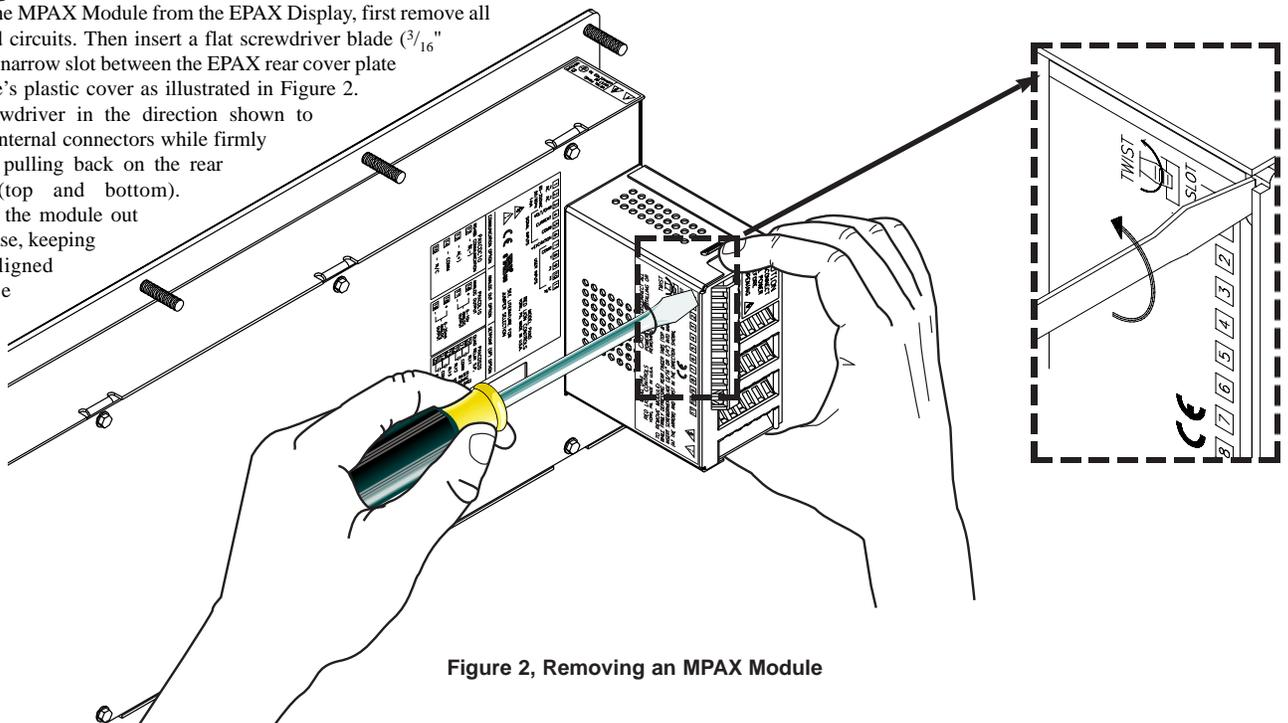
Figure 2, Removing an MPAX Module
