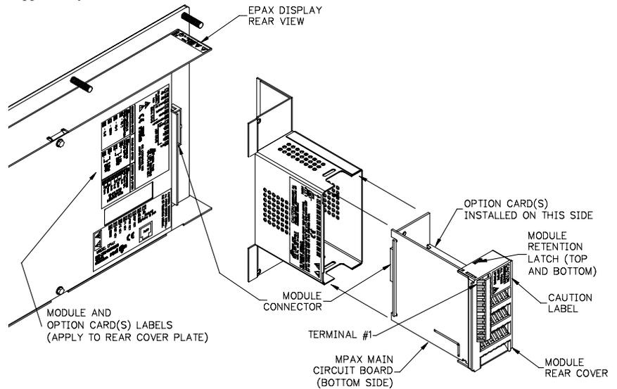
Figure 1, Installing an MPAX Module and Option Cards
