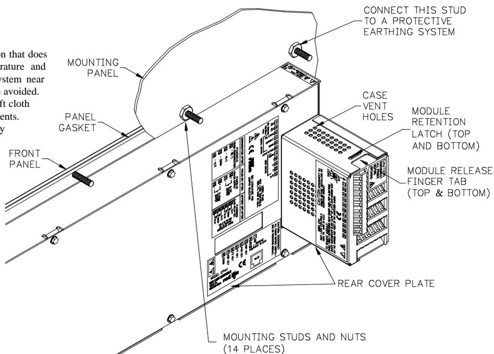
Figure 4, Installing The EPAX Into A Panel
