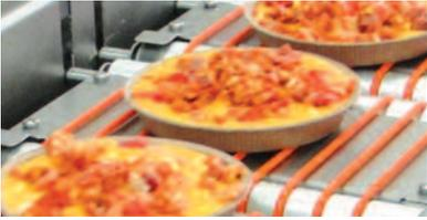
“Like all the best machine designs the principle is simple. This means we are able to easily adapt it or add in some extra capabilities for specific applications,” explains Matt. “For the quiche job, the collator is actually made up of three smaller independently controlled conveyors.”
