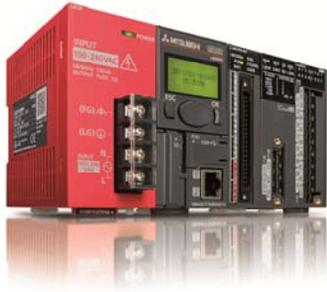
**Picture 2:** Every MELSEC L series PLC CPU provides 24 I/Os, a 2-channel high speed counter, 2-axis positioning, pulse catch and interrupt functions. The built-in communications options include an Ethernet port, providing a simple interface to higher level control systems.
