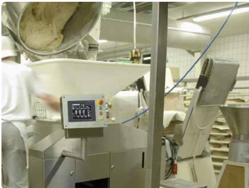
Variable speed and servo control technologies provide accurate scaling of the dough
