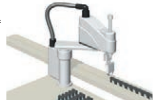
Example: Palletizing of loads using a SCARA robot
