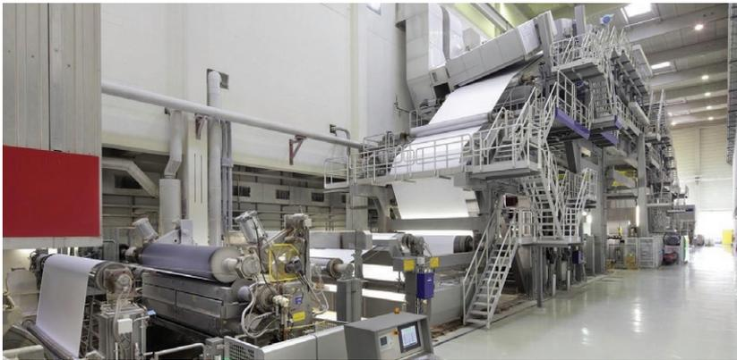
Thermal paper gets its characteristics from a special coating. It is typically used for sales receipts and tickets. At the Mitsubishi HiTec Paper plant in Bielefeld, Germany (MPEB), around 300 tonnes of thermal paper goes through one of the coating machines every day.
