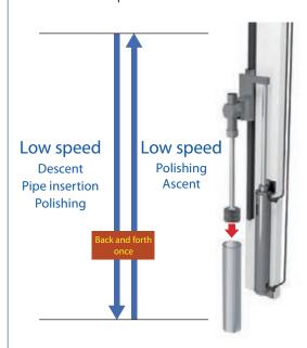
To ensure that the necessary quantity is produced and to ensure product quality, the ascent and descent during polishing are performed at low speeds, and cannot be performed more than once.
