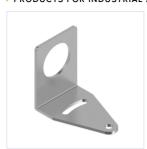
Bracket: Right Angle Mounting Material: 12 Gauge Stainless Steel Curved mounting slot for versatility/orientation Clearance for M6 (1/4 in.) hardware Part Number: 32723
