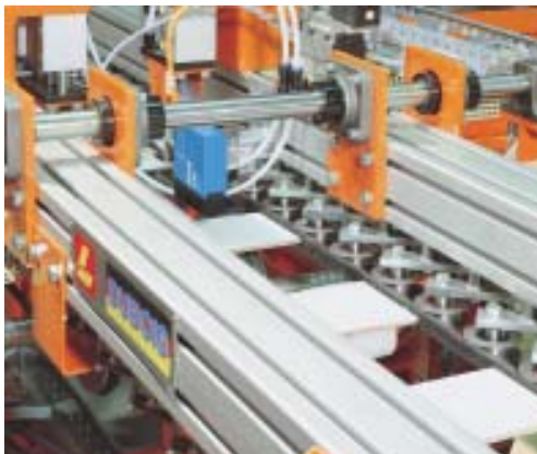
▲ Once a fluorescent marking has been applied during quality control, tiles can be sorted automatically into quality categories using a luminescence scanner.
