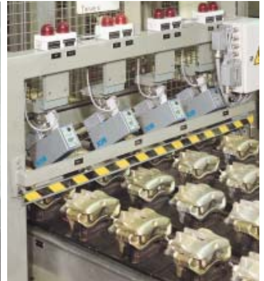
▼ LUT 1-4 luminescence scanners used to ensure that brake callipers for vehicles are correctly fed in.
